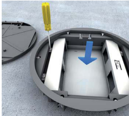
2 | Device insert, plastic, round Place device insert into round plastic installation unit from the top and tighten firmly using four thread-rolling screws.
